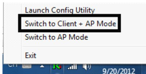
This mode lets you use the adapter both as a Soft-AP and client at the same time. Switching to this mode, you can let a wireless adapter be connected to a wireless network (Soft-AP) with Internet connected, and let others adapter be indirectly connect to Internet via the Soft-AP wireless network.
