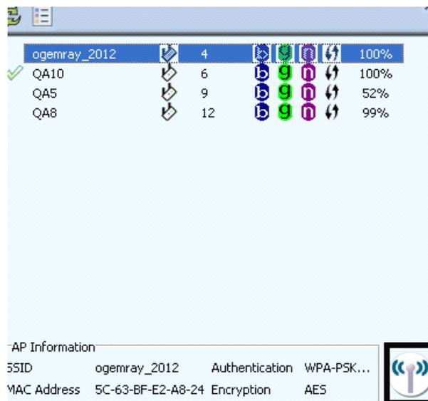
5. The Ralink Utility automatically detects and displays the security settings of the network to which you are connecting in the Profile Settings screens. If the Utility shows that WPA-PSK or WPA2-PSK security is detected as shown below, click the right arrow to save your settings.
