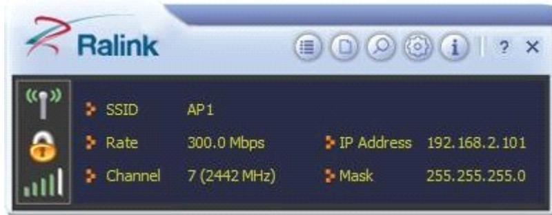
The Ralink wireless utility starts in compact mode as shown above, provides profile management, the available networks listing, a statistical counter display, Wi-Fi multimedia (WMM), protected Wi-Fi setup, Cisco compatible extensions (CCX), call admission control (CAC), radio controls, Ralink driver/utility information, and help
